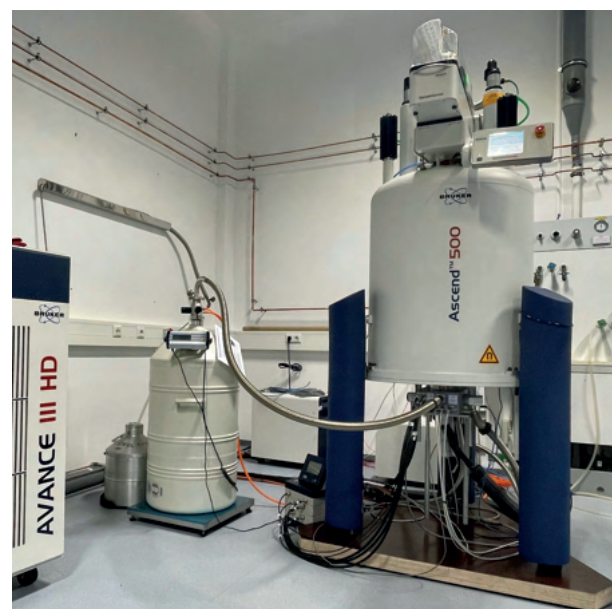
A Bruker Avance III HD 500 MHz spectrometer with Prodigy cryo-probe (-40 to +70 °C) is used for NMR investigations. The probe allows the acquisition of 1D and 2D spectra of most relevant nuclei (1H, 19F, 13C, 15N, 29Si, 31P, ...)
